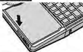
When closing the disk cover, press down near the drive power/open switch (position of the arrow) to ensure that the cover is locked.
